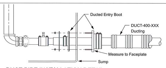
**DUCT PIPE INSTALLATION DETAIL**
