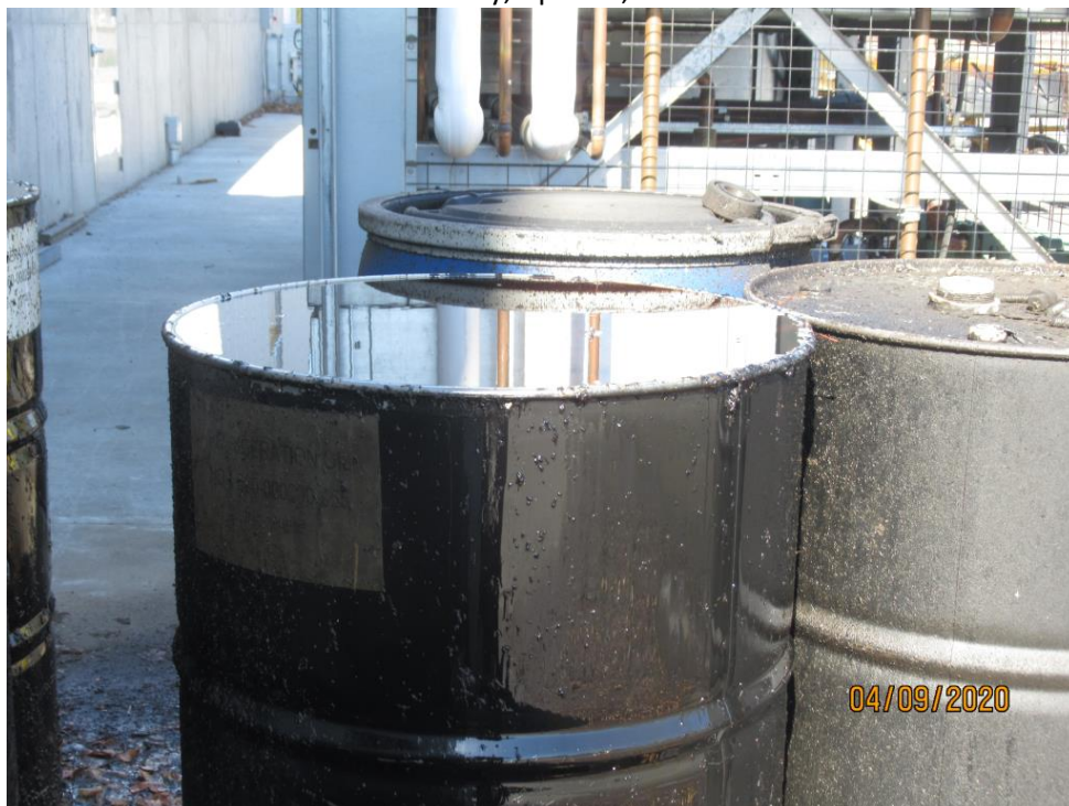
Photograph 47 :Refrigeration oil drums, note oil pooling on the top and leaking around the sides.
