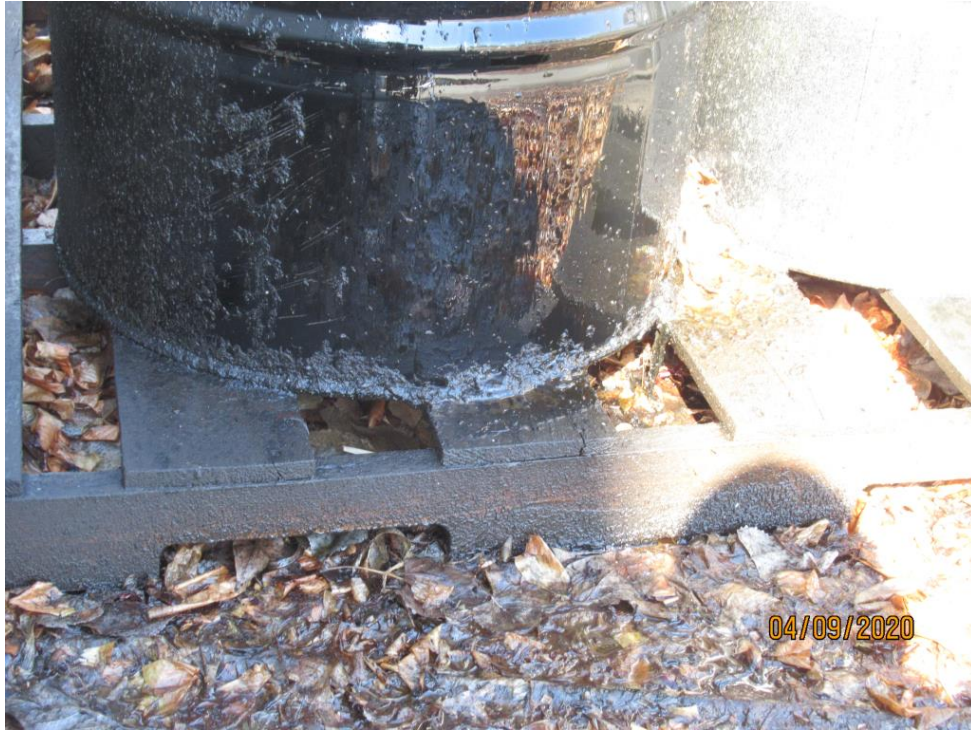
Photograph 49 :Leaking oil from refrigeration oil drums on to storage pallets.
