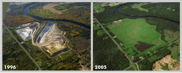
Aerial photo of Flambeau open pit mine before and after successful backfill operation PHOTO: Applied Ecological Services
